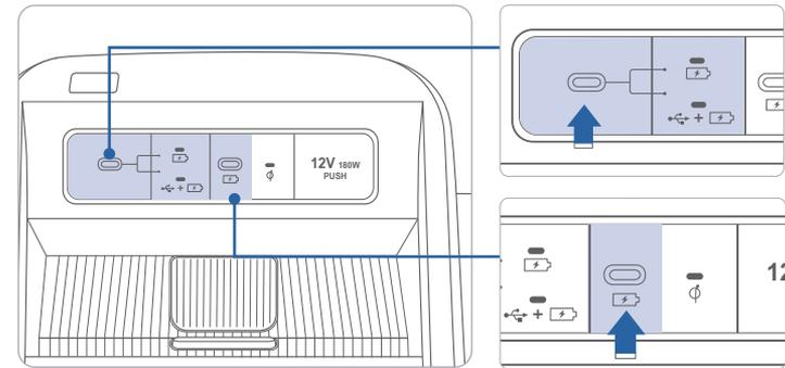
The left port can be set for USB data or charging only, by pressing the switch. The icon on the switch will illuminate for the mode selected.
