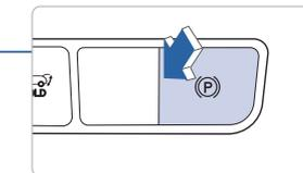
Press the EPB switch while depressing the brake pedal.
