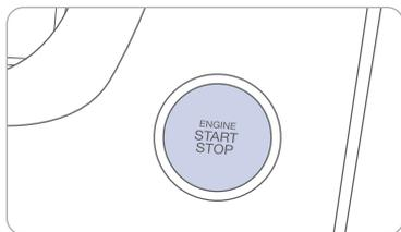
With the ignition OFF and foot OFF of the brake pedal, press the Engine Start / Stop button.
