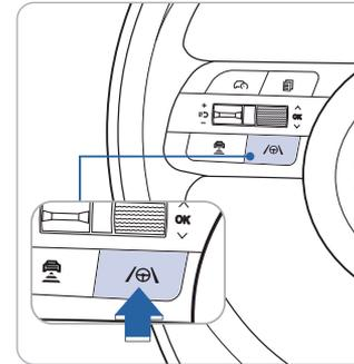
Lane Keeping Assist is designed to help detect lane markings (or road edges) while driving over a certain speed. The system will warn the driver if the vehicle leaves the lane without using the turn signal, or will automatically assist the driver's steering to help prevent the vehicle from departing the lane.
