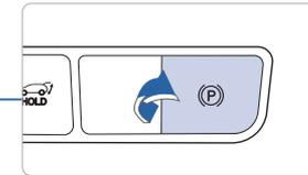
Stop the vehicle then pull the EPB switch.
