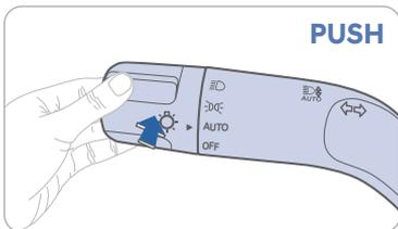
High Beams will automatically activate when headlights are set to AUTO. To override pull back twice on the lever.
