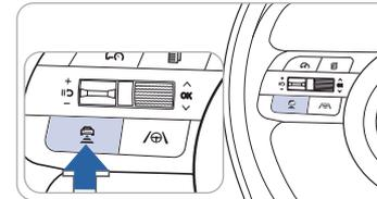
Smart Cruise Control allows you to program the vehicle to help maintain a constant speed without holding the accelerator pedal, while maintaining a consistent distance with the vehicle ahead.
