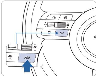
Lane Following Assist helps detect lane markers on the road using the front view camera mounted on the front windshield. LFA helps to assist the driver steering to help keep the vehicle centered in the lane.
