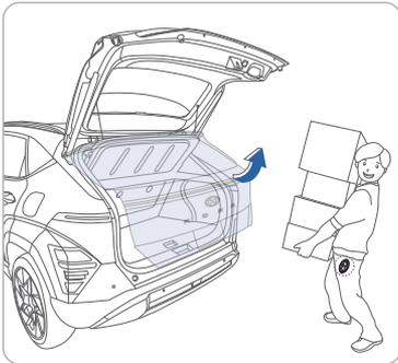
On vehicles equipped with Smart Liftgate, the liftgate can be opened with no-touch activation.
