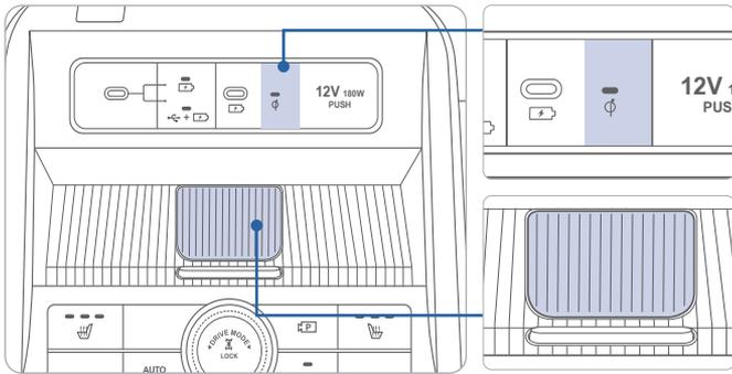
There is a wireless cellular phone charging pad in the center console. The system operates with all doors closed and the ignition in the ON position.
