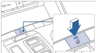
Press the heated steering wheel button to warm the steering wheel. The indicator on the button will illuminate. Press the button again to turn the heated steering wheel off.
