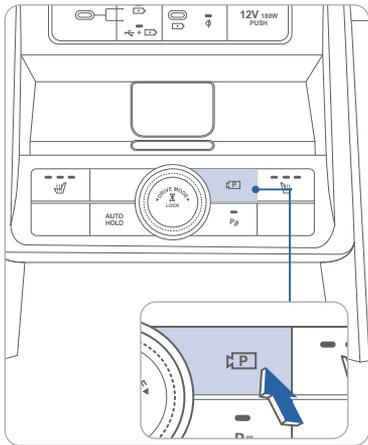
Rear View Monitor displays the area behind your vehicle to help with parking or driving.
