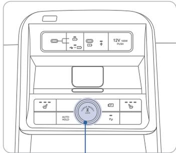
The mode changes, as below, whenever the DRIVE MODE button is pressed. An indicator will illuminate on the instrument cluster when the vehicle is in sport mode or smart mode. When the vehicle is in comfort mode, it is not displayed on the instrument cluster.
