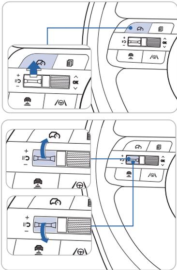
1. Press and hold, for 3 seconds, the Driving Assist (Ⓛ) button at the desired speed. The Speed Limit (LIMIT) indicator will appear on the instrument cluster.
