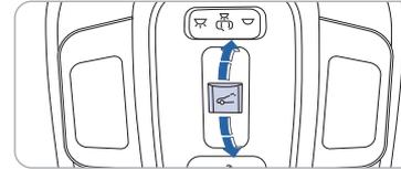
Push the sunroof control switch backward to the second detent position. First the power sunshade will open and then the sunroof will open automatically. push the sunroof control switch forward to the first detent position to close the sunroof only. push the sunroof control switch forward to the second detent position to close both the sunroof and the power sunshade automatically.
