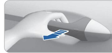
**To Unlock:** Place your palm behind the door handle and grip the door handle. It will unlock as you pull the door open.
